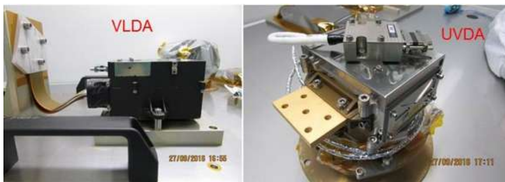
Fig. 13. Detector units at delivery at the Optical Payload Systems facility at ALTEC in Turin. The two cameras, VLDA, and UVDA are mounted face down on the transport plates.
