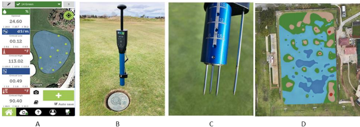
Figure 1. The POGO TurfPro (Stevens Water Monitoring Systems; Portland, OR, USA) system utilizes a POGO Pro+ turfgrass insight sampling tool, and a bluetooth-linked mobile application (TurfPro Mobile) for data collection and analysis. A: Example of data collection and analysis output from putting green #14 on a golf course; the image indicates the perimeter of the site (i.e., putting green, left image), the location of the current nine sampling sites taken so far within that putting green, soil moisture (percent volumetric water content), soil electrical conductivity ( \text{dS}\cdot\text{m}^{-1} ), surface heat index (as ^{\circ}\text{C} or ^{\circ}\text{F} ), salinity concentration index ( \text{dS}\cdot\text{m}^{-1} ), and root zone temperature (as ^{\circ}\text{C} or ^{\circ}\text{F} ); the spatial analysis is completed on an Amazon Web Services hosted platform in sync with the mobile application that turfgrass managers utilize. B: POGO TurfPro hand-held wireless device or meter commercially called POGO Pro+. C: POGO TurfPro soil moisture measuring components (5.6 cm [2.2 inch] length metal rods on an integrated sensor apparatus) on left-side of image; single metal rod on right-side of image measures soil temperature. D: An example of the spatial analysis of moisture content across a football pitch.
