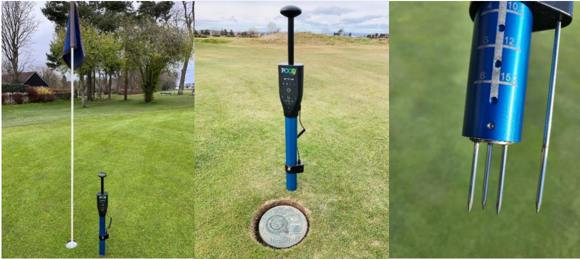
Figure 1. The POGO TurfPro (Stevens Water Monitoring Systems; Portland, OR, USA) is a portable device equipped with 5.6 cm metal rods that measures soil volumetric water content to the 5.71 cm depth. The extended metal rod at right side of device measures soil temperature.
