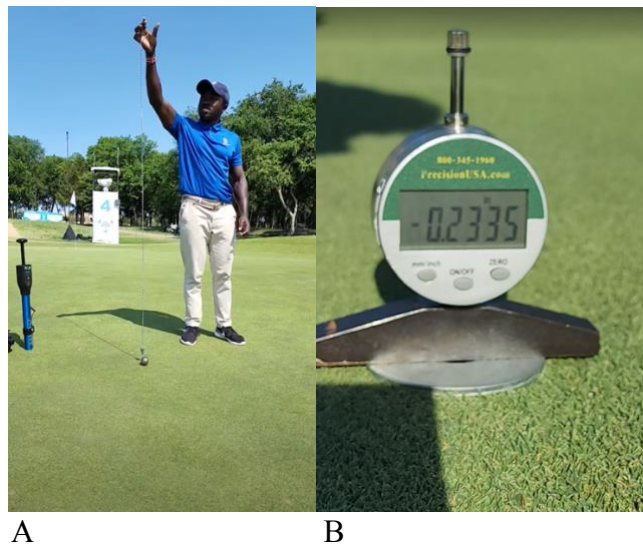
Figure 3. Example of measuring putting green surface firmness using the Precision Putting Green Firmness Compaction Meter (Precision USA; Pompano Beach, FL, USA). A: Dropping a weighted ball from an exact 1.8 m (6 feet) height to the surface. B: Measuring the depression formed in the turf surface.
