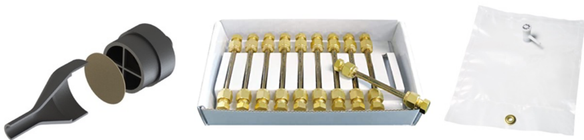
Figure 5: Elements of the sampling system; starting from the left PM filter, desorption tubes (Photo by RESTEK) and sampling bag (Photo by RESTEK).
