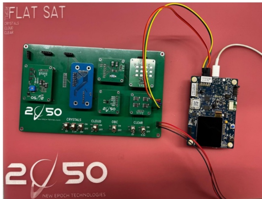
Figure 6: FlatSat after first integration.
