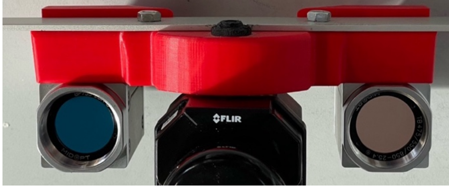
Figure 3: Basler cameras with internally mounted filters (C-mount).
