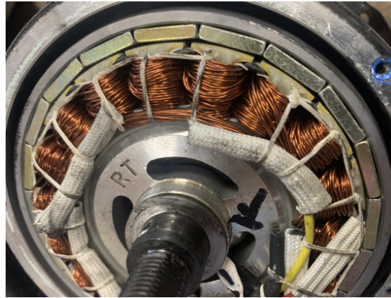
Figure 16. SPM motor in a wheel hub (18-slots/20-poles configuration).
