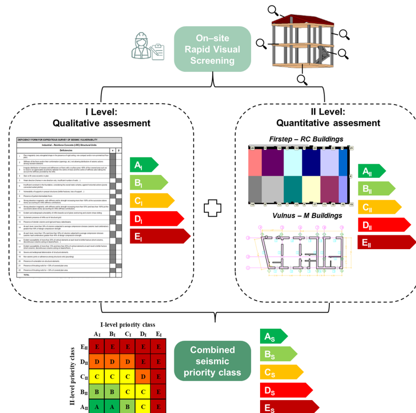
Figure 5. Illustration of the adopted seismic priority-based ranking procedure.
