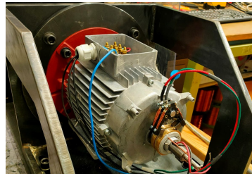
Figure 13.9: HEPM motor prototype. Sliding contacts can be noted.
