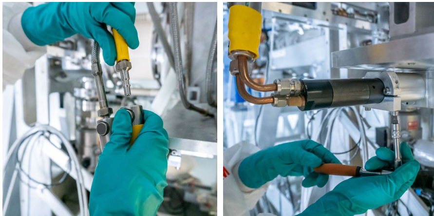
Figure 6.19: Pneumatic motor installed on the SPES Front-End; (left) unplugging of the pneumatic connections, (right) opening of the fastening clamp.
