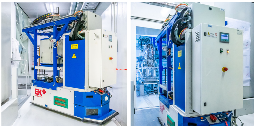
Figure 3.16: The Horizontal Handling Machine (HHM) during commissioning tests nearby the SPES Front-End.
