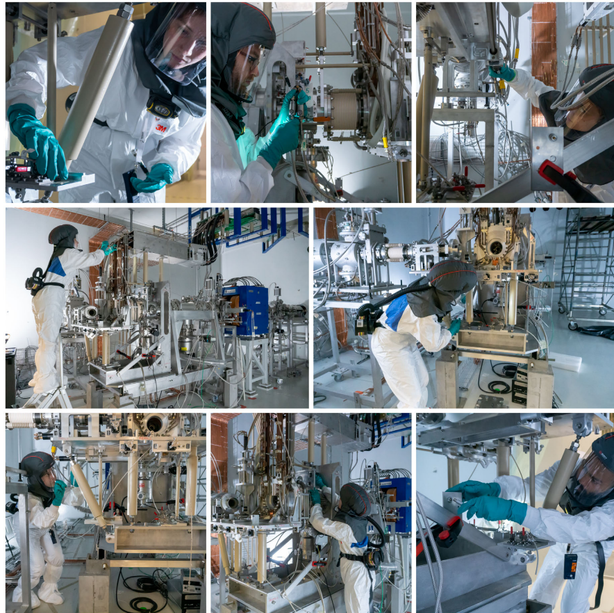
Figure 6.7: Different examples of SPES Front-End maintenance tests.
