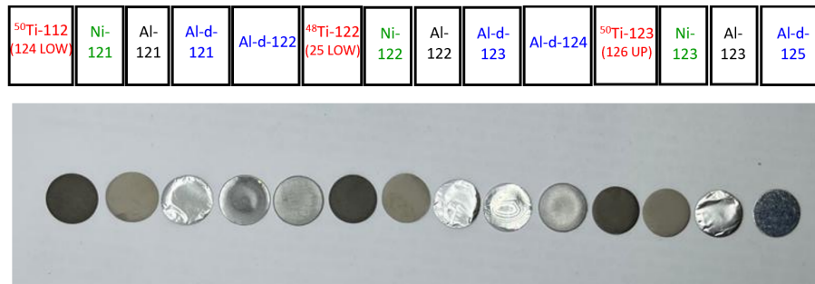
Figure 3.8: Configuration of the stacked-foils target irradiated in the 12 th experiment of the REMIX project. The repeated sequence of enriched Ti foil (names in red), nat Ni monitor foils (names in green), thin nat Al catcher foils (names in black) and thicker nat Al degrader foils (names in blue) can be seen.
