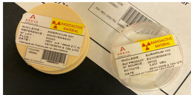
Figure 3.19: ^{152}\text{Eu} and ^{241}\text{Am} point-like sources used for the efficiency calibration of the HPGe detectors.
