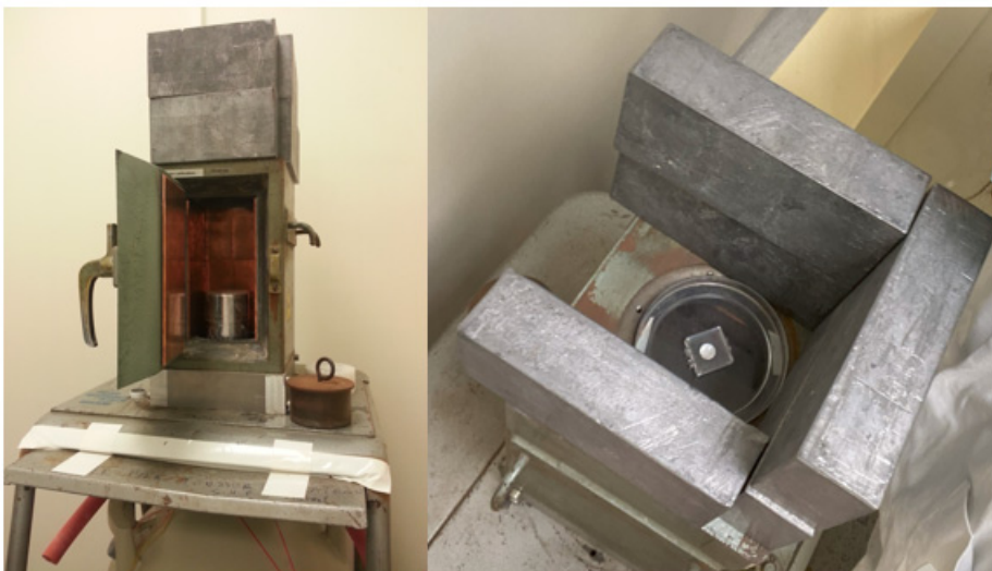
Figure 3.17: First HPGe detector used for measurements: front and top view. Positioning of the target is at 19 cm far from the detector surface, shielded by lead blocks.
