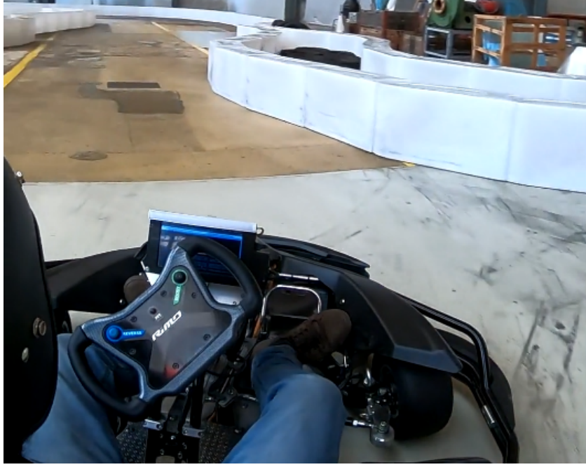
Figure 9.11. The real go-kart platform driving autonomously.
