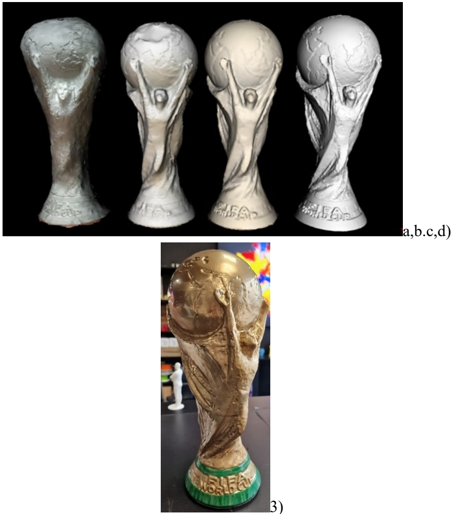
Figure 66 Word Cup Scanned by a) LiDAR b) Photogrammetry c) Structured Light scanner with 1 mm of resolution d) Structured Light scanner with 0.5 mm of resolution and e) Final model.
