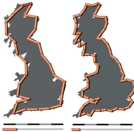
Figure 28 An example of the coastline paradox. If the coast of Great Britain is measured using units 100 km long, the length of the coast is about 2,800 km. With units of 50 km, the total length is about 3,400 km, about 600 km longer [56].
