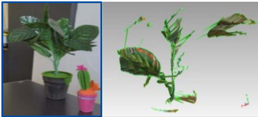
Figure 23 Reconstruction of artificial plant using low-cost RGB-D camera Intel Real Sense.
