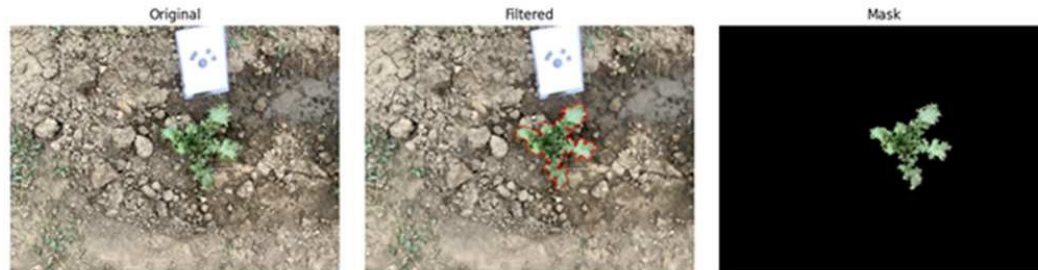
Figure 131 leaf area recognition process. Left panel: original image. Central panel: filtered image after the application of RGB threshold and weed removal routine. Right panel: Final result of the segmentation algorithm.
