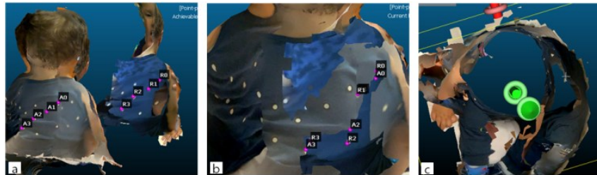
Figure 144 Example of LiDAR scans alignment: a) point selection for alignment; b) alignment; c) top view of alignment.
