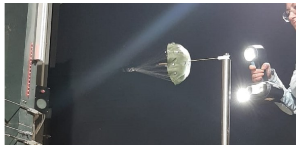
Figure 19 Parachute scanned with Structured Light system
