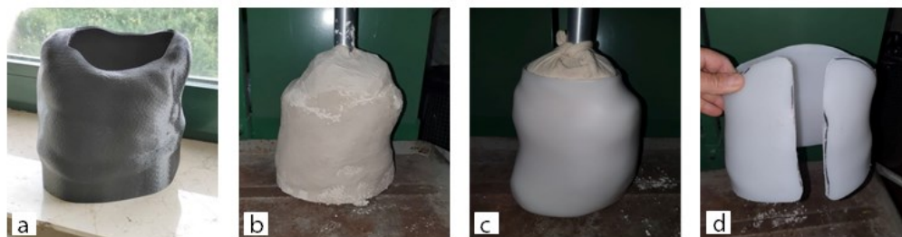
Figure 150 a) 3D printed trunk, b) Plaster mould built on printed model, c) Plaster realization d) Final model.
