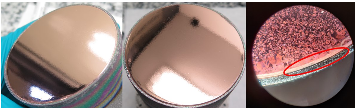
Figure 6.43: Ultimate photos of the QPR B4 sample and the defective spot
