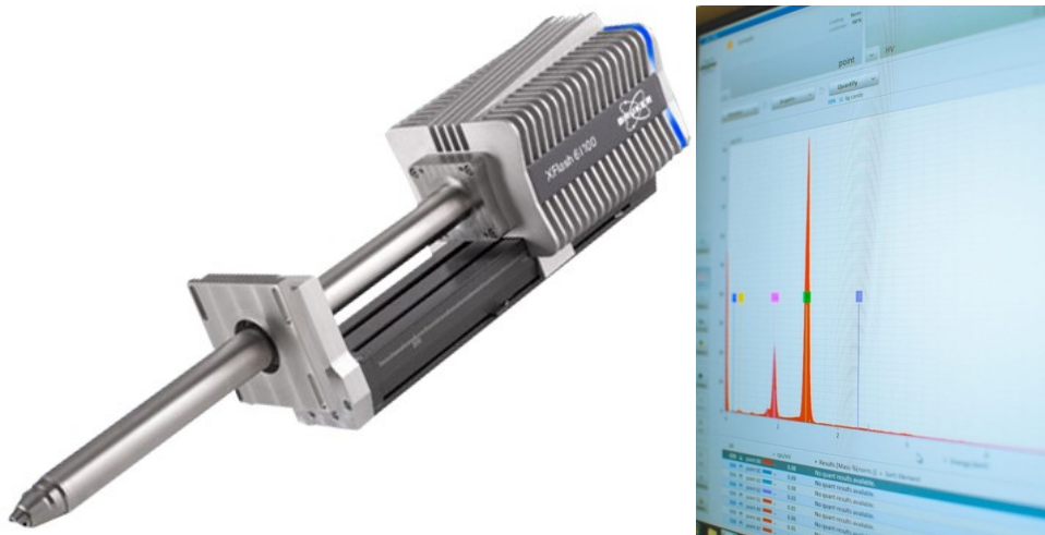
Figure 4.4: Image of the Bruker EDX module and a supplied software for EDX spectroscopy analysis
