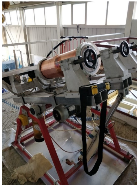
Figure 2.14: A tumbling system at the Legnaro National Laboratories of INFN
