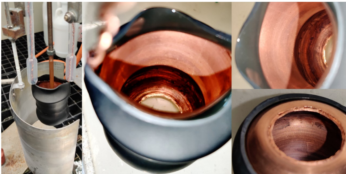
Figure 6.33: Photo of the double-cathode system, isolation and dummy substrate
