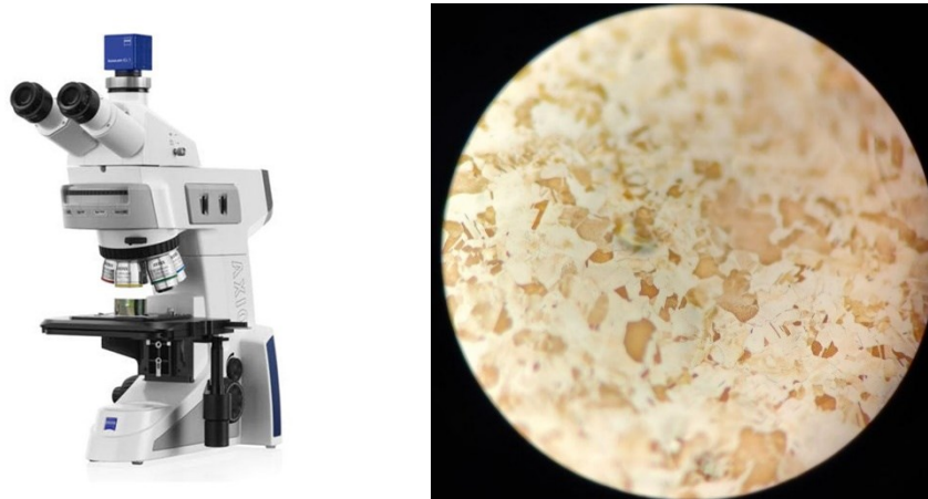
Figure 4.5: An Axio Lab.A1 microscopy and the typical output of the analog surface photo
