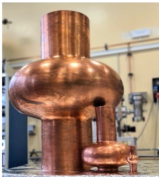
Figure 2.7: Spinning formed resonant copper cavities: 500 MHz, 1.3 GHz, 6 GHz
