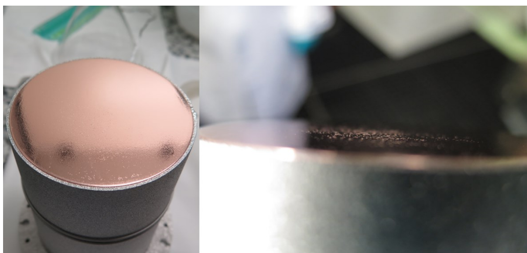
Figure 6.42: Photo of the QPR B4 sample after stripping
