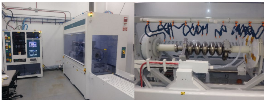
Figure 2.25: New improved horizontal EP system at Jlab [126]
