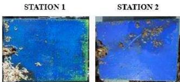
Fig. 9. Examples of antifouling activity of paint Sailing pro with 38% of copper (I) oxide: station 1 (low hydrodynamics); station 2 (highest hydrodynamics).
