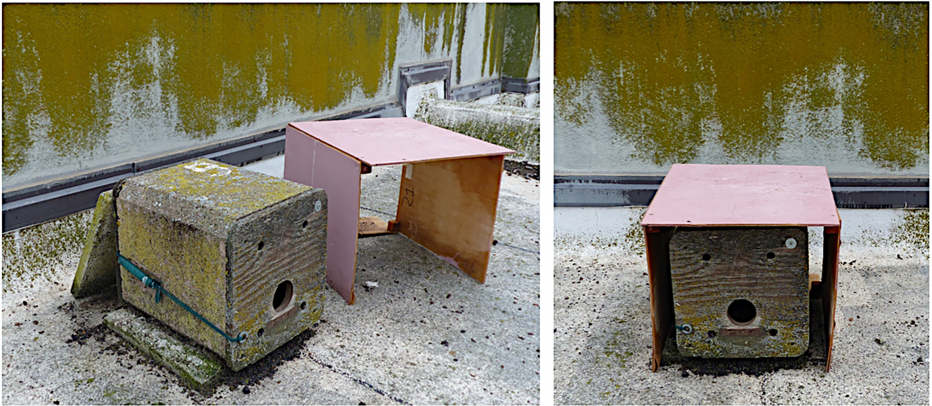
FIGURE 1 Left panel: control nest box with shading cover on the side; right panel: shaded nest box, with the shading cover preventing direct sunlight exposure while allowing air to flow on both sides and top of the nest box. The quarry tile that was used to shade the rear wooden panel (on the internal side of which the temperature logger was attached) is also visible behind the nest box in the left panel. The wall fencing the experimental roof terraces, which prevents nestlings from falling down the terraces when abandoning their nest box, is visible on the background.
