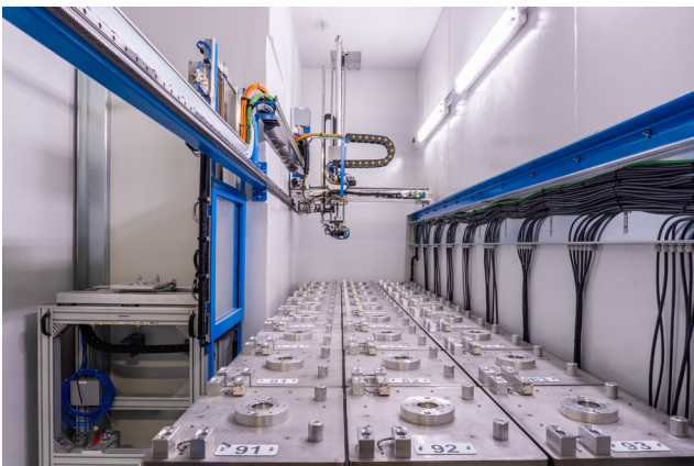
Fig. 1. The TSS cartesian manipulator and the storage rack designed to host up to 54 TIS units.
