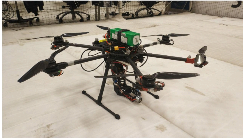
Figure 1.3.: Example of an aerial robot composed of an hexarotor with a 2 d.o.f. arm.
