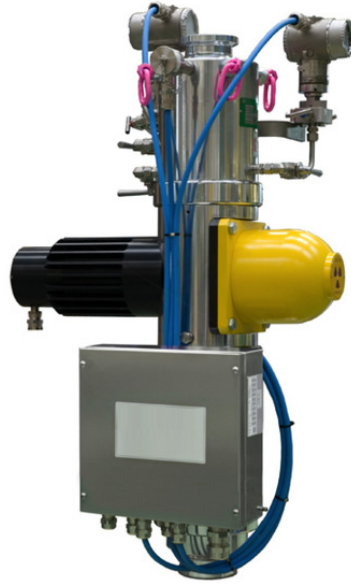
Figure 2: A Multiphase Flow Meter built in a modular way: it is possible to observe the Venturi tube placed in vertical position with the pressure probes and the densitometer placed in horizontal position. The impedance probes are installed inside the tube in close contact with the fluid.
