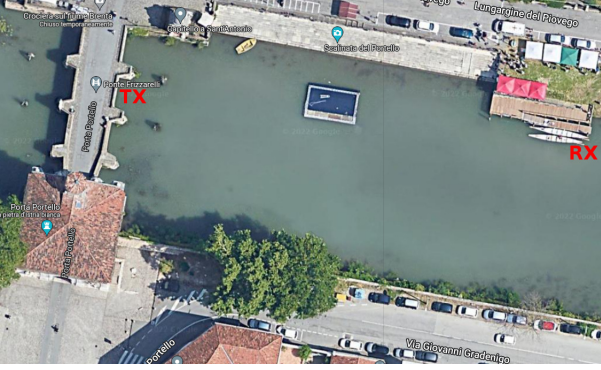
Fig. 3: Picture of the testing area. The transmitter (left) was deployed from the Portello bridge, while the receiver (right) was deployed from a service jetty. The distance between transmitter and receiver was 80 m.
