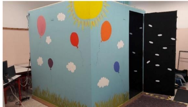
Figure 3.1. Experimental room. The room measured 2 x 2 meters and was soundproof, with black interior walls and equal numbers of white clouds randomly fixed on each wall. The external walls were painted with a child-friendly landscape which was designed to encourage children to enter
