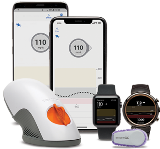
Figure 1.1: Example of the Dexcom G6 systems, including the CGM sensor, and the auto-applicator, together with devices which allow the real-time monitoring of CGM values and trend.
