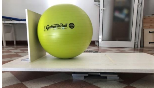
Figure 3.3. Dynamometric platform expanded with the wooden board.
