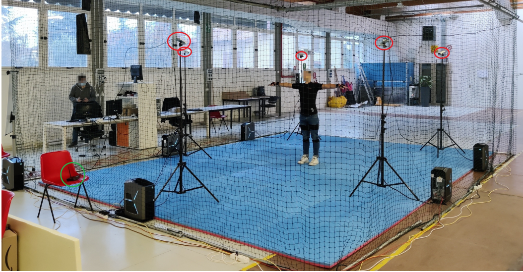
Figure 4.2: Experimental setup used for the acquisition of the UNIPD-BPE dataset. The five RGB-D cameras are highlighted in red, while the inertial suits' master receiver is highlighted in green.
