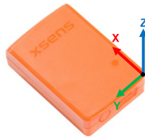
Figure 3.2: Xsens MTw Awinda and its default local coordinate reference system (source: [132]).
