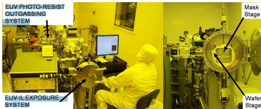
Figure 4.17: Extremely Ultraviolet Interference Lithography (EUV-IL) at Center for NanoTechnology, University of Wisconsin-Madison, Madison, WI, USA 53706 [163]
