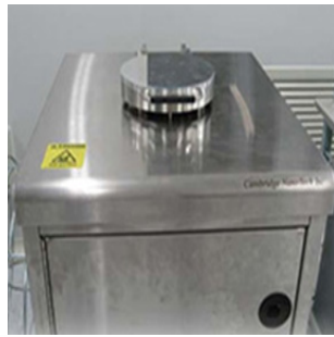
Figure 4.6: (a) The working principle of ALD, (b) Savannah-100 ALD system in the laboratory of Microfabrication, Institute of Physics, CAS [156]
