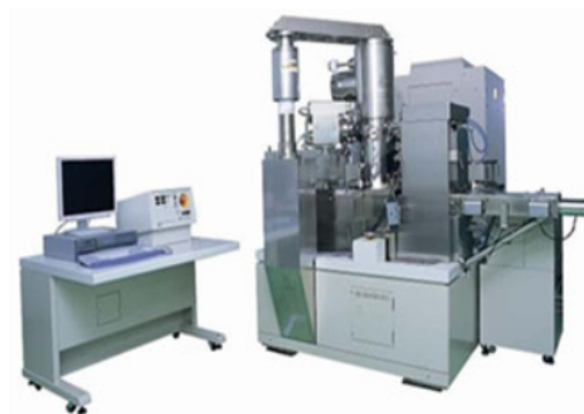
Figure 4.13: Electron beam lithography system JBX-6300FS, the laboratory of Micro-fabrication, Institute of Physics, CAS [156]
