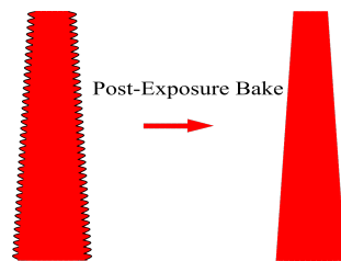
Figure 4.3: The function of post-exposure bake
