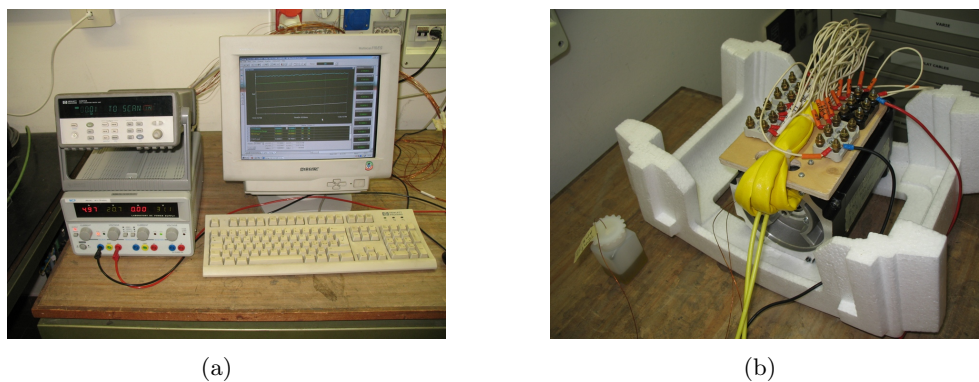
Figure 7.29: Thermal test: (a) acquisition system and DC current supply, (b) motor under test and oil box for ambient temperature.
