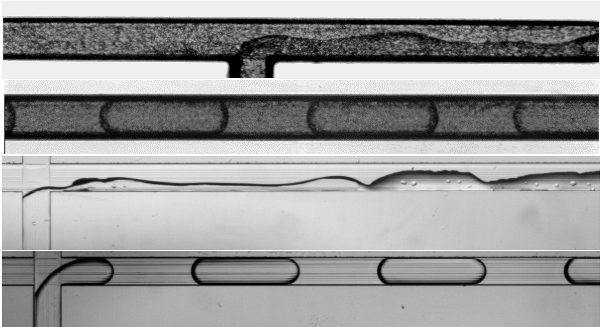
Figure 4.15: Effect of the functionalization on the production of droplets. Starting from the top the micrographs refer to: the laser ablated T-junction before the functionalization process, and the same T-junction generating droplets after the functionalization; the cross-junction obtained with the DISCO DAD 321 dicing saw before the functionalization and the same generating droplets after it was functionalized. As can be seen in both cases droplets cannot be generated without tailoring the wetting properties of the channels surfaces.
