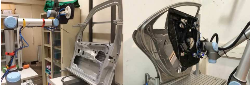
Figure 8.9: The robot is able to insert the plastic module into the door, both in Stuttgart and laboratory facility.
