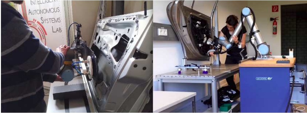
Figure 8.6: The robot is physically guided to follow the desired motion through Kinesthetic Demonstration.
