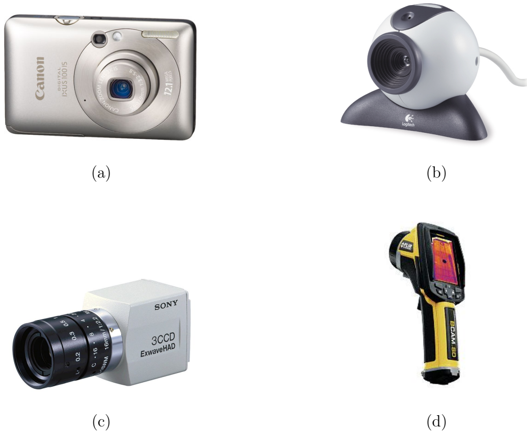
Figure 3.1: Some type of digital cameras : (a) A consumer CMOS photo camera; (b) A cheap CMOS webcam; (c) An industrial CCD camera; (d) An infrared thermal imaging camera.
