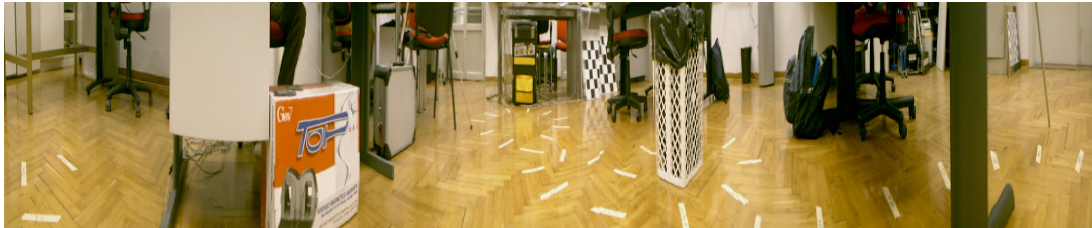
Figure 4.3: The 360-degrees panoramic image composed with the automatically stitching procedure by the Kondo KHR-1HV.
