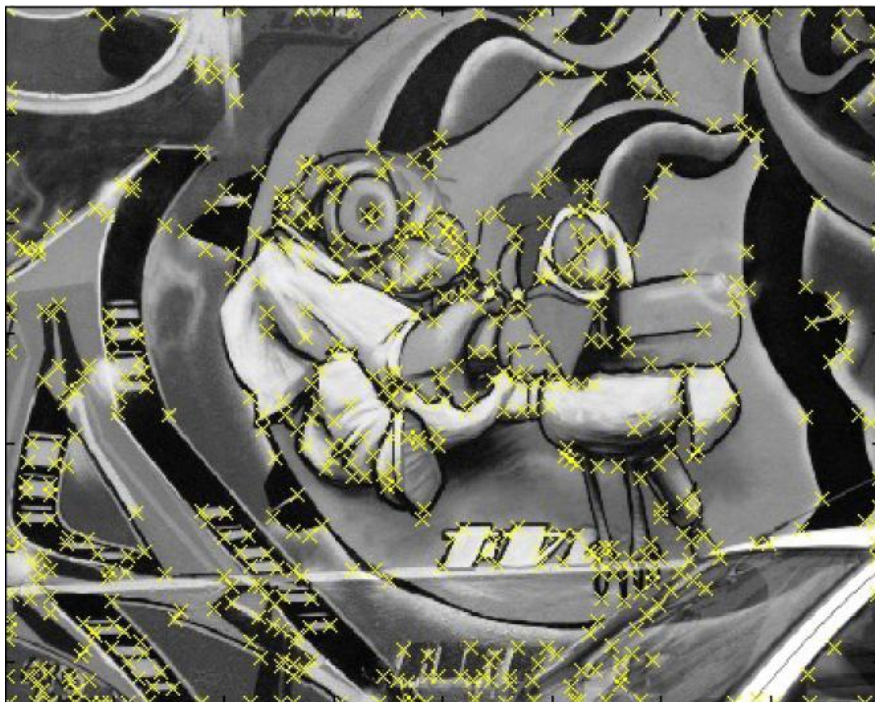
Figure 3.9: The interest point selected by the Harris detector [courtesy of Tinne Tuytelaars].
