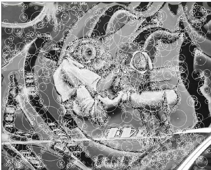
Figure 3.6: The interest point selected by the Difference of Gaussians detector [courtesy of Tinne Tuytelaars].
