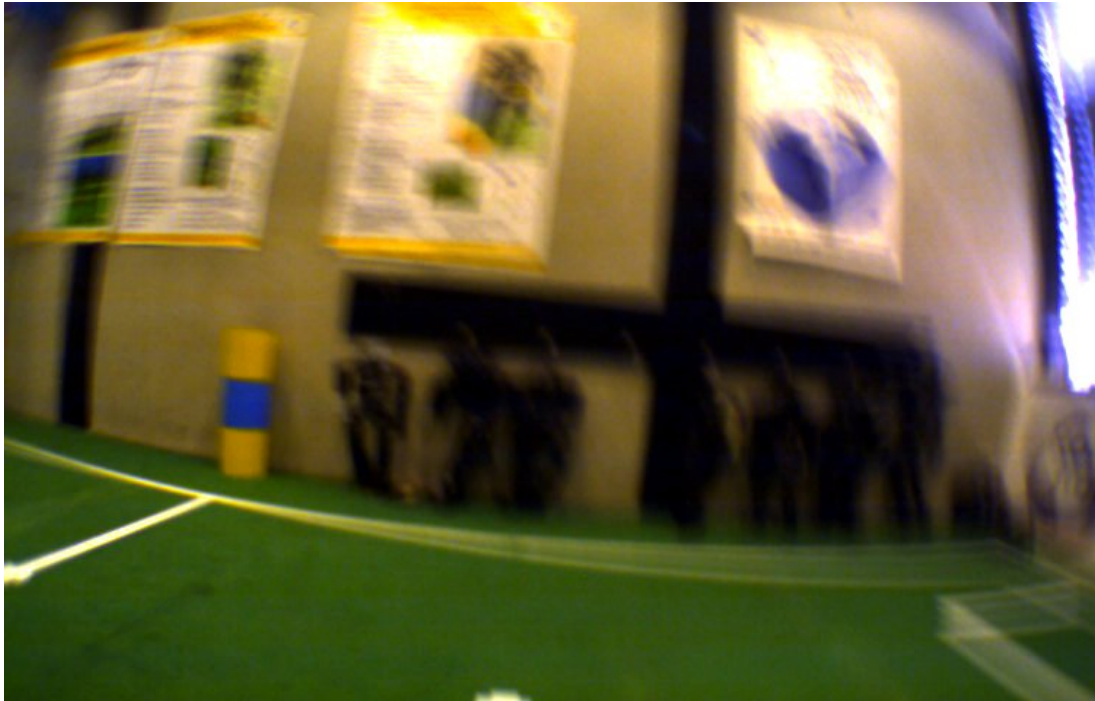
Figure 5.1: Typical image grabbed by a walking humanoid robot. As can be seen, the image is highly affected by motion blur.
