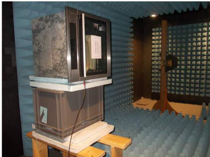
Figure 2.46: A picture of the oven in the anechoic chamber on the rotating support: the configuration reported is for measuring the gain in the yz -plane
