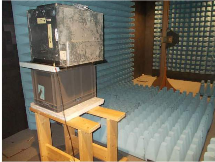
Figure 2.45: A picture of the oven in the anechoic chamber on the rotating support: the configuration reported is for measuring the gain in the xz -plane
