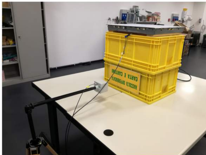
Figure 4.17: Measurement setup for oscillating EM fields around the hob.
