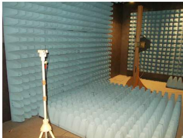
Figure 2.28: The antenna board inserted in the plastic casing in the measurement chamber.
