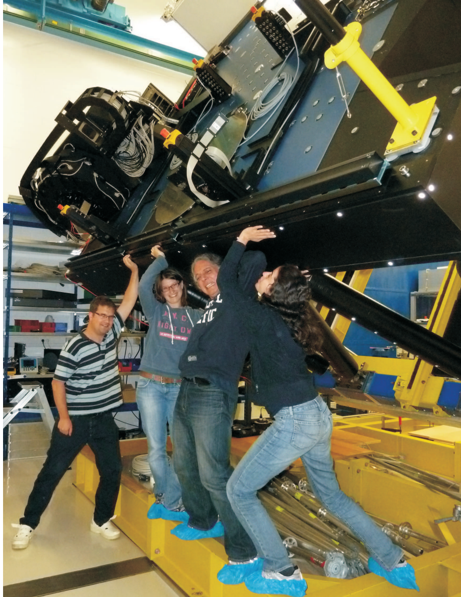
Figure 3.73: A picture of the GWS mounted on the LN bench tilted by 60°.
