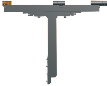
Figure 3.14: The mechanical structure of one SE, supporting the 2 lenses and the pyramid. The T-shaped support is needed to connect the SEs to the GWSs stages.
