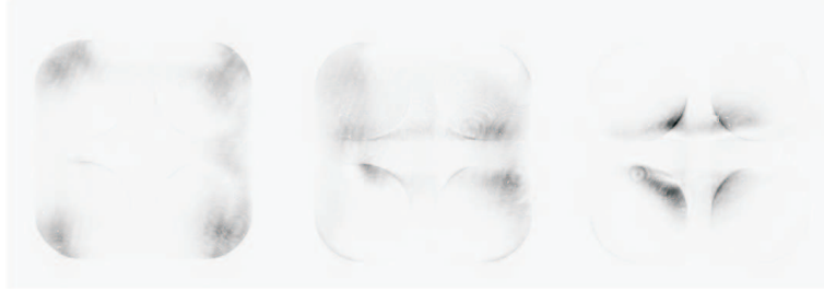
Figure 3.44: Effect of different defocus signals on the four pupils on the test CCD. This effect is amplified because, for alignment purposes, a monochromatic red laser light is used, producing a very small spot on the pin of the pyramid.
