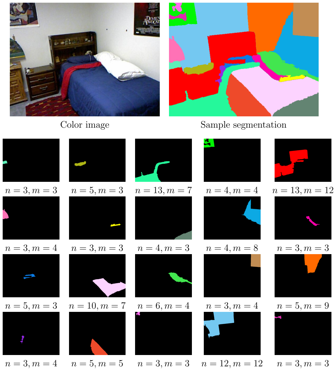
Figure 3.1: A sample segmentation with the binary masks for each region, and the corresponding numbers of control points (in the u and v parametric directions) used for the NURBS surface approximation.
