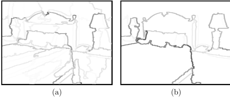
Figure 5.3: Computation of b_{i,j} on a sample scene. (a) b_{i,j} values on the initial over-segmentation. (b) b_{i,j} values on the final result after all the merging steps. The boundary colors are proportional to the similarity between the neighboring segments (dark gray corresponds to low b_{i,j} values, light gray to large ones).
