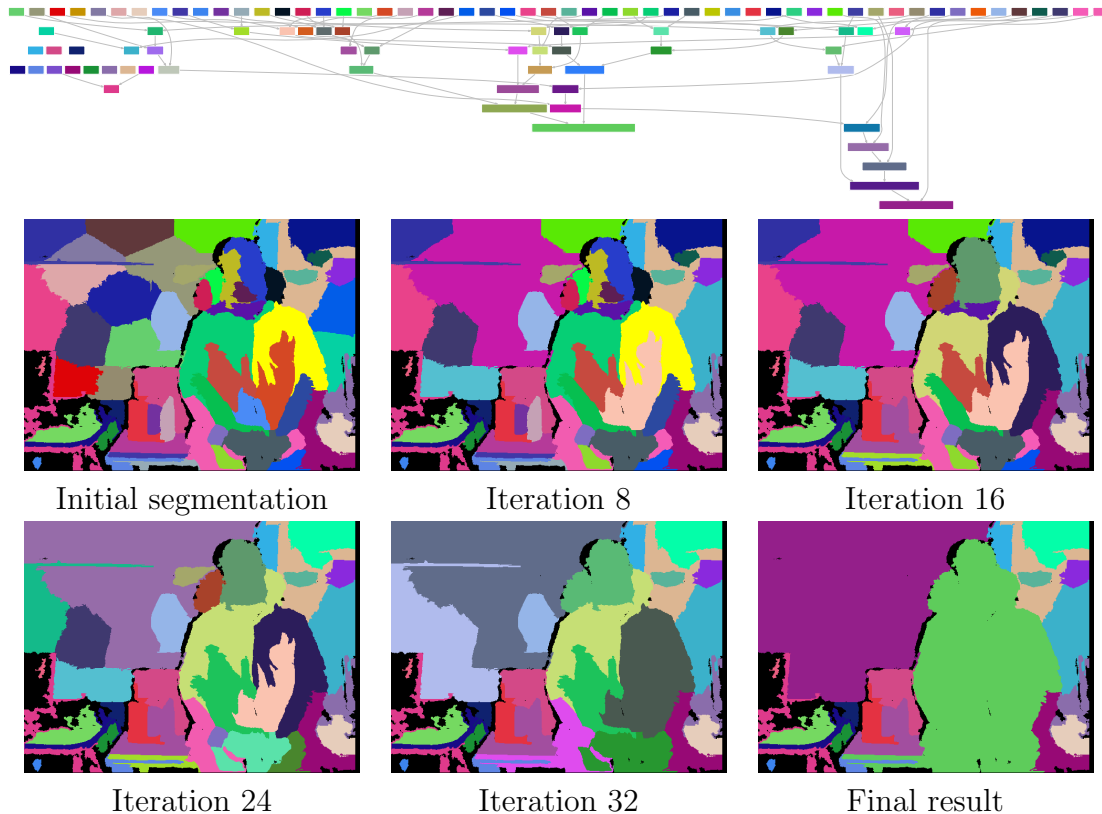
Figure 4.6: Example of the merging procedure on the scene of Figure 4.9, sixth row. The images show the initial over-segmentation, the merging output after 8, 16, 24, 32 iterations and the final result (iteration 41). The graph shows the merge operations between the various segments. The colors in the images correspond to those of the graph nodes.
