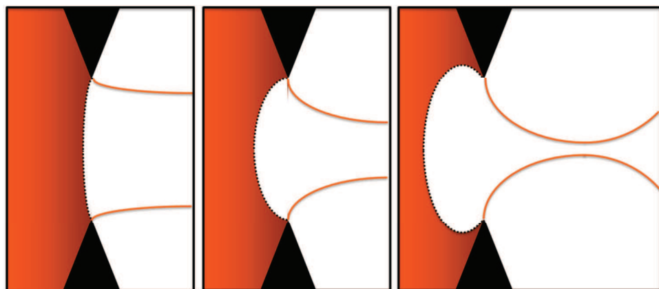
Figure 2.23: Beam profile at different perveance condition. Underperveance (left): meniscus is too flat and the focal point of the trajectories is after the EG. Perveance (centre): meniscus has a correct concave shape and the focal point is inside the EG. Overperveance(right): meniscus concavity is too much and the trajectory focal point is before the EG (hourglass envelope).
