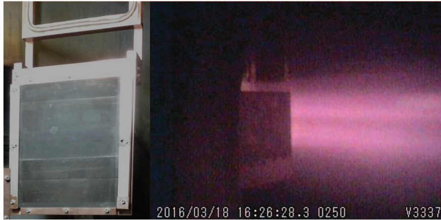
Figure 5.3: (Left) photo of the unidirectional CFC target consisting of 3 CFC tiles with water-cooled copper support frame. (Right) optical image of entire beam passing through the beamline, the upper and the lower beamlet groups are visible in the right part, the retracted copper calorimeter is visible on the left, the CFC calorimeter (also retracted) is barely visible on the upper part of the picture.
