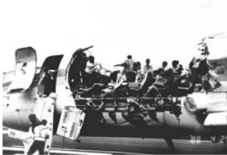
Figure 1.1. Destruction of the canopy due to material fatigue during an Aloha Airlines flight in 1988 (Richard and Sander 2016).
