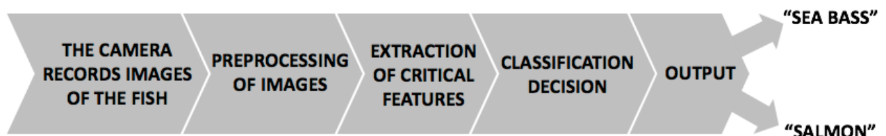
Fig. 1.1 (adapted from Duda et al., 2001). The rough macro-structure of a classification system that could be applied to the described example. First, images of fish examples are recorded. The images (input to the classifier) are then preprocessed in order to make the classification easier (noise elimination), and critical features (those that allow the classification between different species) are extracted from the whole set of physical features. Then the decision about the belonging class (either sea bass or salmon) is taken.
