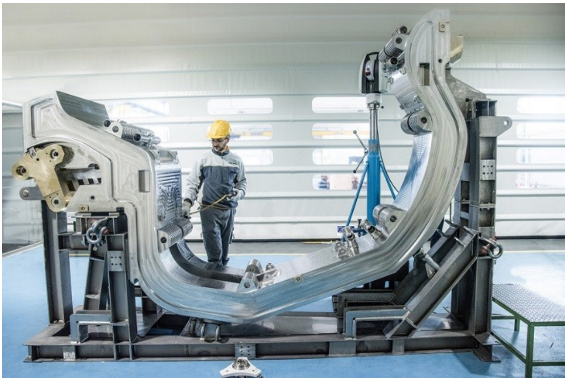
Figure 2.4: European real-size prototype of ITER Divertor Cassette manufactured by Walter Tosto [22].
