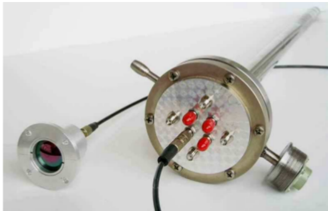
Figure 3.5: Cryostat of the photo sensors Figure 3.6: LLL photo sensors.
