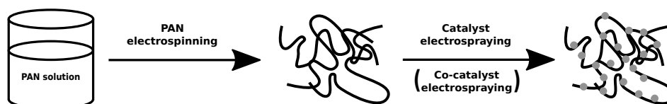
Figure 6.1: Steps for the membranes fabrication by the layer-by-layer approach
