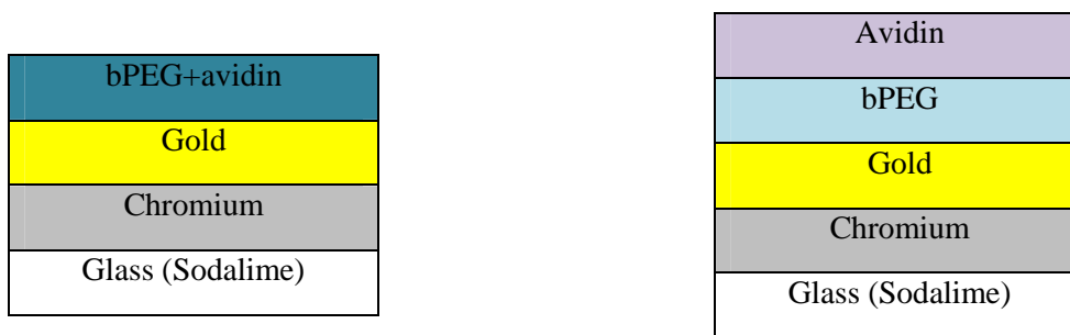
Figure 4. 8. Fitting model scheme for the Single- (left) and Multi- (right) PEO 2/5 kDa. For A and B Cauchy model parameters, values of 1.45 (corresponding to a wavelength of 620 nm) and 0.01 were used respectively.[120]
