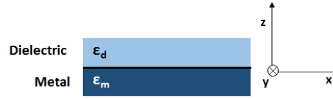
Figure 1.3. Planar metal/dielectric interface.
