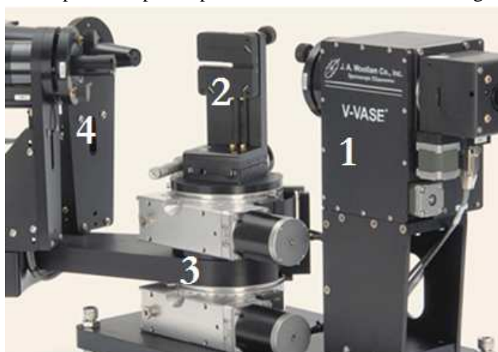
Figure A.1. 2. Picture of the spectroscopic ellipsometer used in this work. (1) Optical bench for focusing and polarization control of the output light (monochromatized by a gating monochromator, located in sequence to a Xe-Neo 75 W lamp), (2) sample holder, (3) rotating goniometer for incidence angle scan, (4) Detector.
