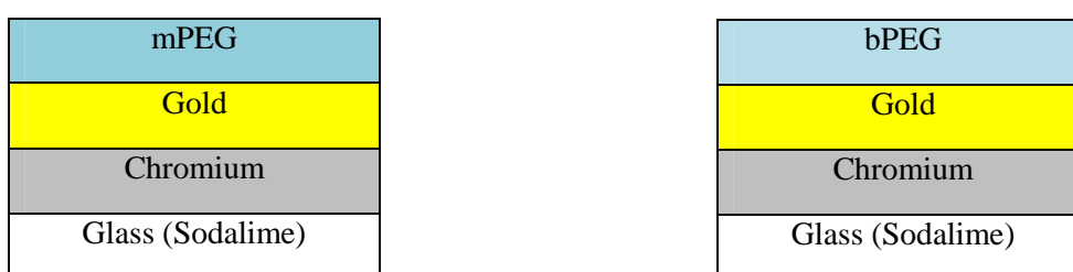
Figure 4. 7. Fitting model scheme for methoxy- ( left ) and for Biotin- ( right ) PEO 2/5 kDa. For A and B Cauchy model parameters, values of 1.45 (corresponding to a wavelength of 620 nm) and 0.01 were used respectively.[120]
