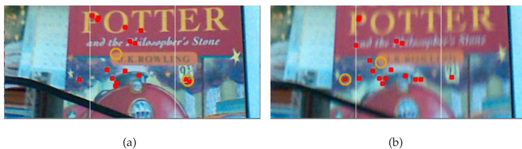
Figure 5.9. Example of correct matches in presence of motion blur: above, a zoom of an image grabbed by the robot without motion blur, below the image grabbed while moving, thus with motion blur.
