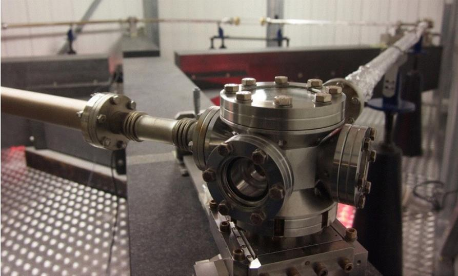
**Figure 1.9:** Detail of a corner mirror of the GINGERino experiment at LNGS
