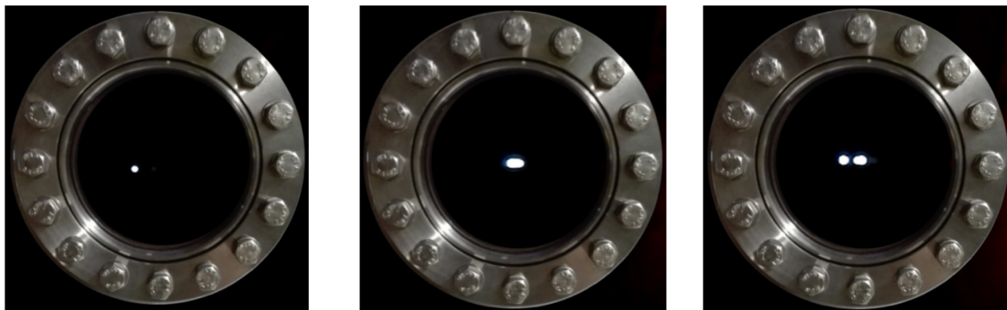
Figure 6-12 – Pictures of sparks between the electrodes (frame extracted from video, the flange was added to figure out the position of the sparks)
