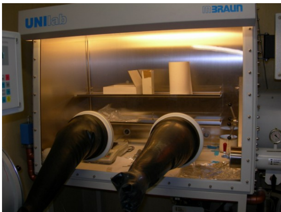
Fig. 24 – Glove box used for the manipulation and storage of uranium compounds.
