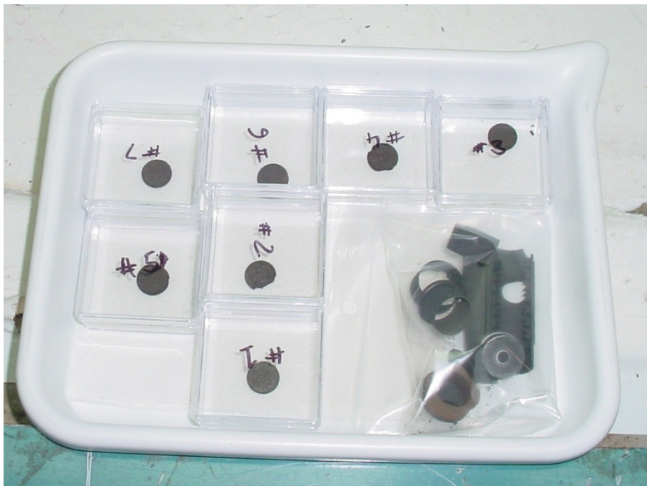
Fig. 60 – Seven “low density” \text{UC}_x discs after the online test.
