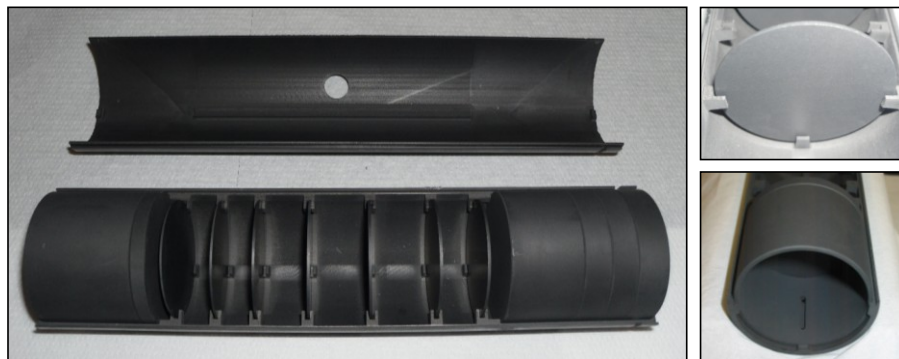
Fig. 13 –SPES graphite box loaded with 7 SiC discs and graphite dumpers and windows [5].
