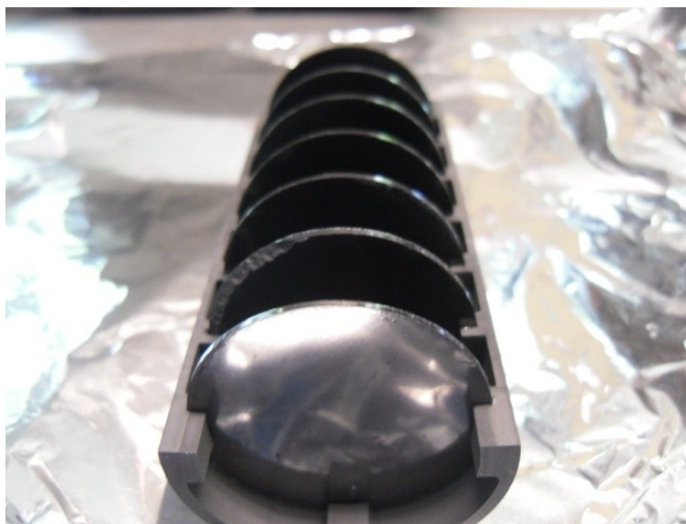
Fig. 78 – Seven green \text{La}_2\text{O}_3/\text{C} pellets placed in a graphite box.
