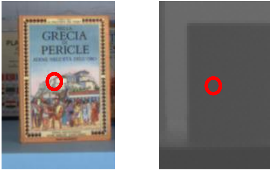
Figure 5.12: Point far from scene distance discontinuities considered in the analysis of the ToF model.
