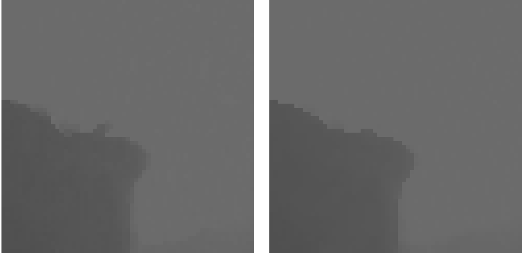
Figure 5.22: Particular of the estimated depth-map with ML (left) and with MAP (right) approaches. The application of LBP improves the quality of the estimated depth-map.
