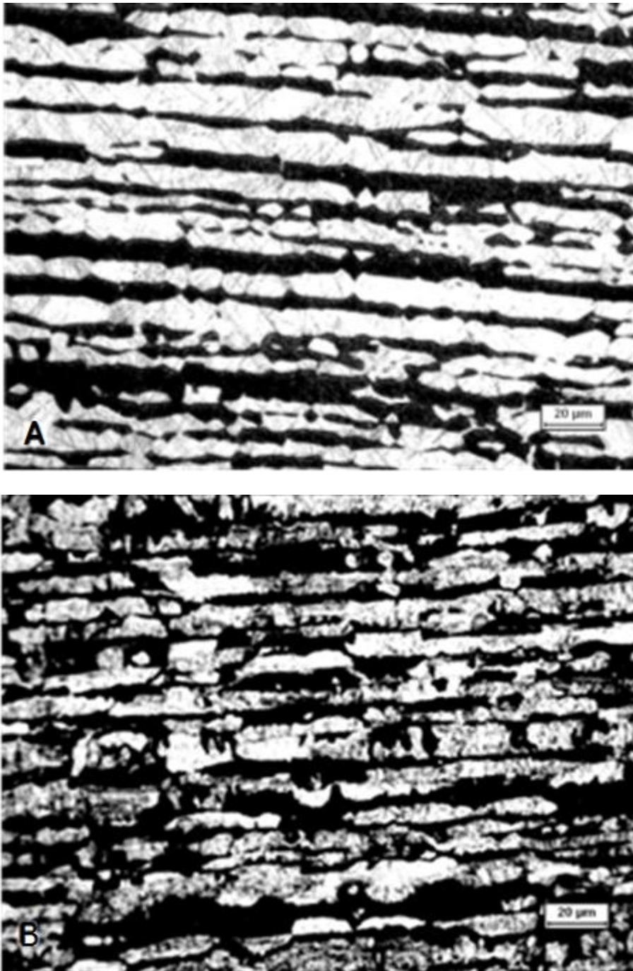
Figure 6.8 Microstructure of cold rolled 2205 duplex stainless steel: a) 10%, b) 85% cold rolled deformation
