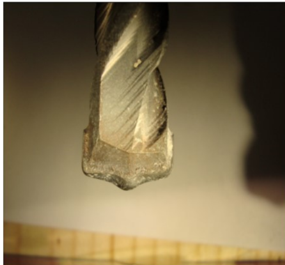
Figure 2.41 Bit 2 after drilling 15.24 m (Condition 2).
