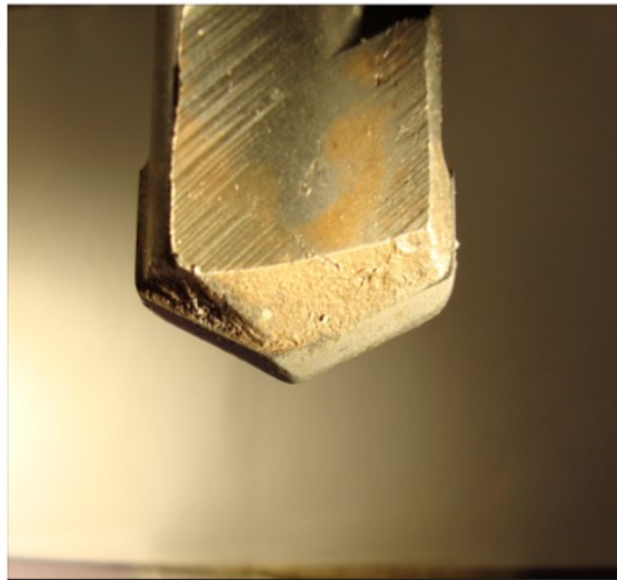
Figure 2.37 Bit 1 after drilling 7.62 m (Condition 1).
