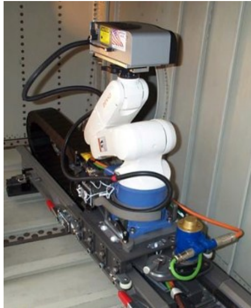
Figure 3.13 Autonomous Maintenance Robot AMR (Krasny 2012).
