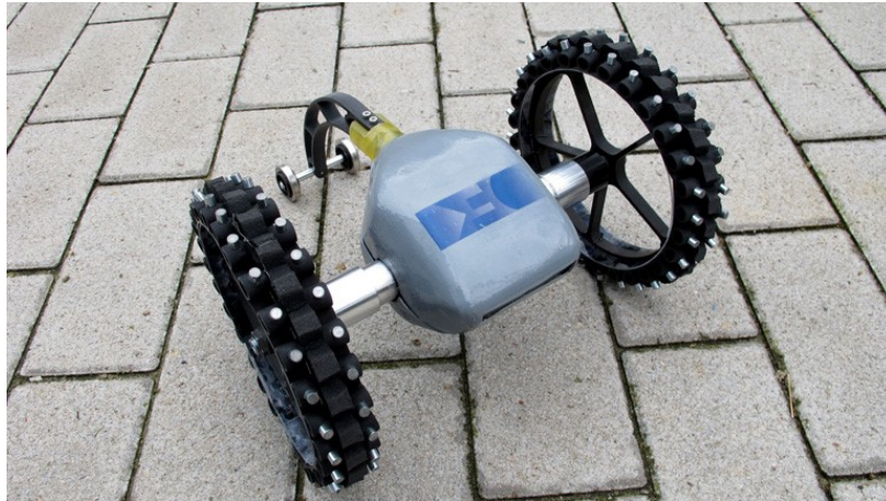
Figure 3.12 Lightweight magnetic climbing robot (Eich & Vogele 2011).
