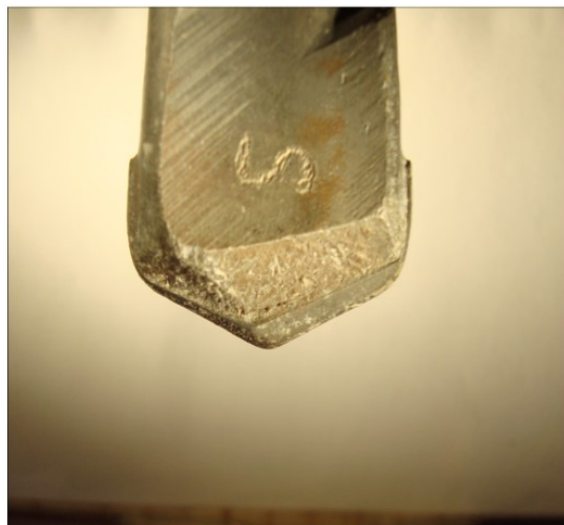
Figure 2.38 Bit 1 after drilling 38.10 m (Condition 5).
