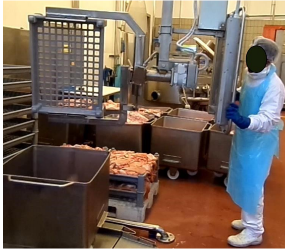
Figure 2.46 Tray unloading with the semi-automatic manipulator.
