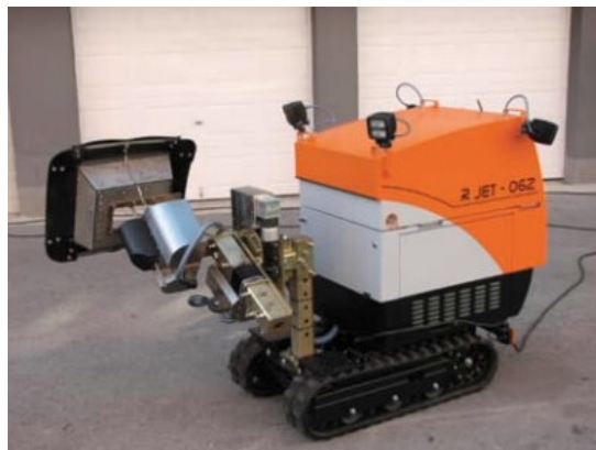
Figure 3.6 Light-weight mobile robot for concrete and metal surfaces (Kovacic et al. 2010).
