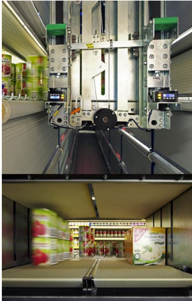
Figure 2.11 WITRON SRS Self Replenishment System (WITRON b).
