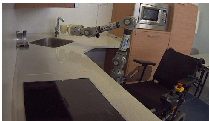
Figure 2.13 The robot assisting a disabled user (Correal et al. 2006).
