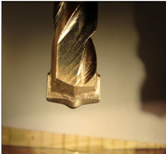
Figure 2.40 Bit 2 after drilling 7.62 m (Condition 1).
