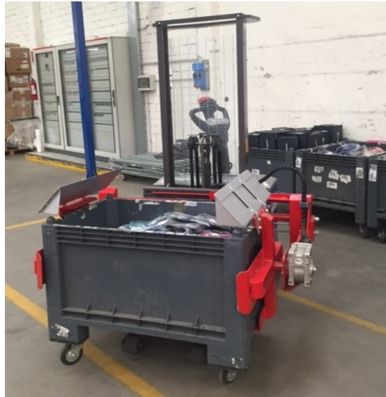
Figure 2.50 Semi-automatic lifting and handling device with lateral barriers.
