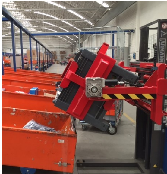
Figure 2.49 Semi-automatic handling and lifting device in the sorting area.
