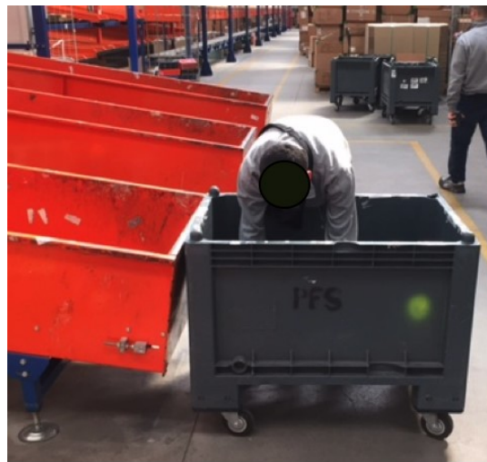
Figure 2.48 Manual worker performing cart emptying.
