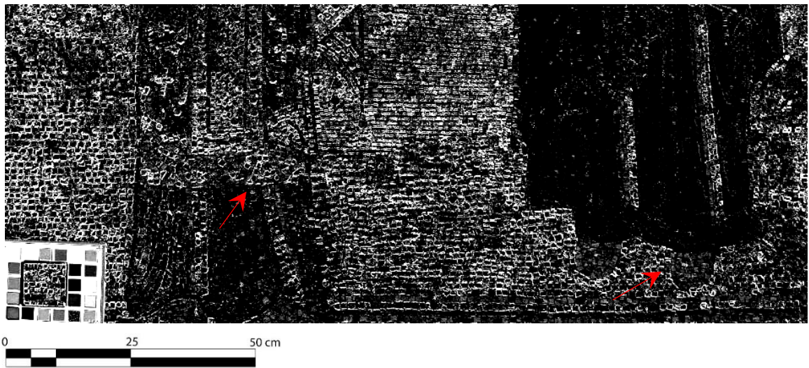
Figure 53. Result of subtraction between visible and infrared non-elaborated images, using Adobe Photoshop. Fragment of the bottom part of the Coronation scene. The red arrows indicate the presence of discontinuities which may help in locating possible stitches of the mosaic fragments.
