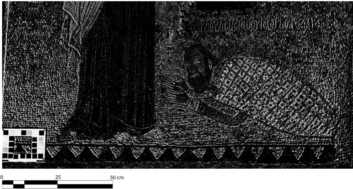
Figure 52. Result of Difference function, applied to the non-elaborated visible and infrared images, by the means of ImageJ. Fragment of the Dedication scene.
