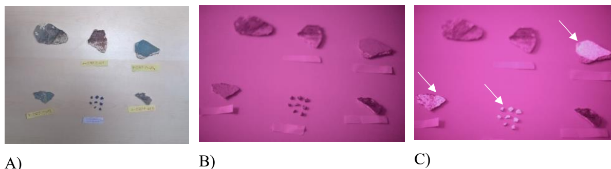
Figure 94. Visible induced infrared fluorescence mode, IR2 bandpass filter. a) Visible light image; b) Near-infrared (IR2) image under natural light conditions; c) Near-infrared (IR2) image when illuminated by a fluorescent lamp (T8 fluorescent tube). The arrows indicate the wall painting fragments with the painting layer containing different concentrations of Egyptian blue.
