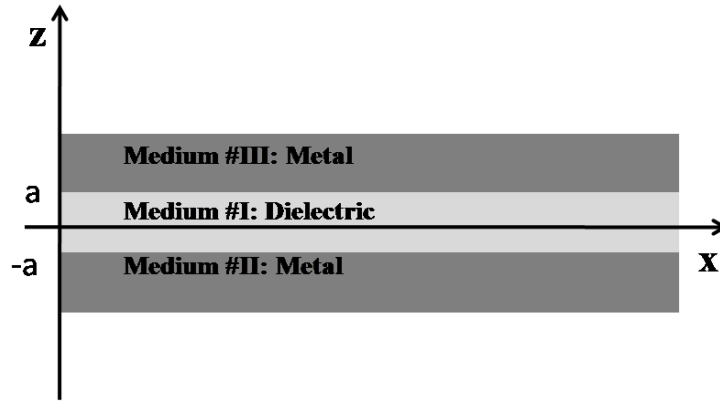
Fig. 1.5: schematic representation of a Metal Insulator Metal (MIM) interface.
