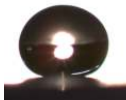
Figure 4.19. 4 \mu\text{L} water droplet on the superhydrophobic copper sample.
