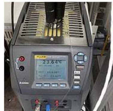
Figure 4.25. (Left) Thermocouples alignment with vacuum inside the section and water in the cooler. (Right) Fluke 9142 calibration bath.
