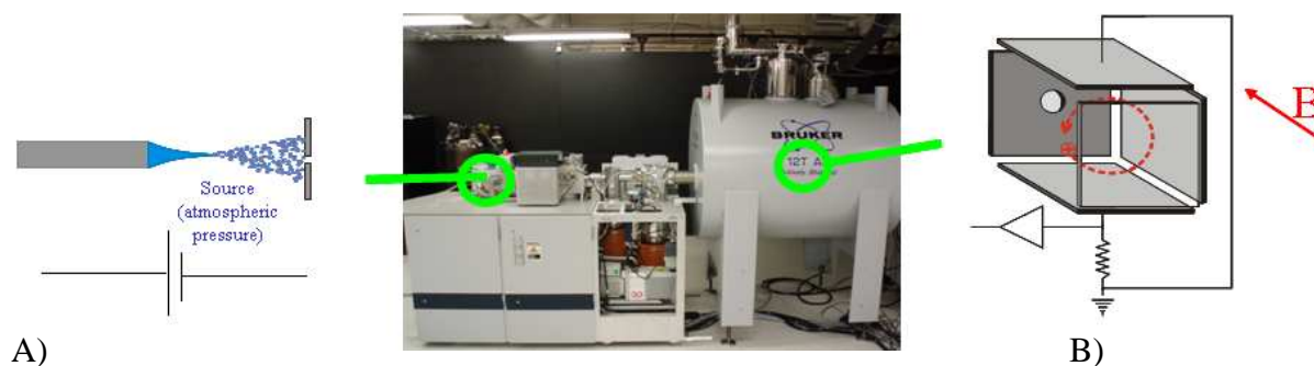
Fig. 16 - Bruker Daltonics (Billerica, MA) Apex IV FTICR. A) Scheme of electrospray. B) ICR cell.
