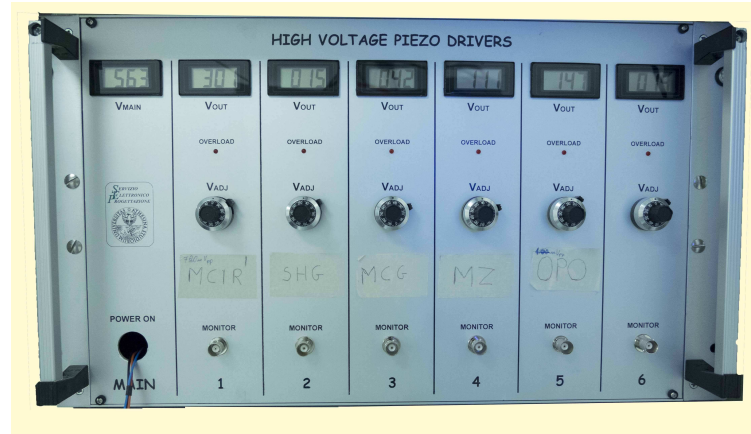
Figure 7.11: Box that contains six high voltage amplifiers
