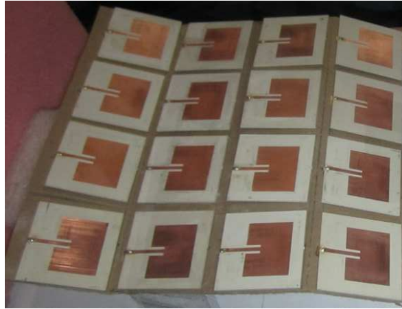
Figure 2.17: Fabricated 4 \times 4 array prototype.
