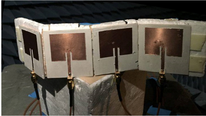
Figure 2.12: Prototype of the fabricated S-shaped array.
