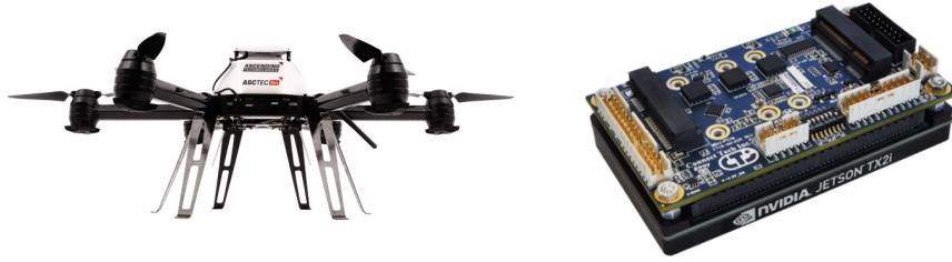
Fig. 3: Left: a multirotor UAV. Right: the Jetson TX2 embedded board that can be easily installed on an UAV.
