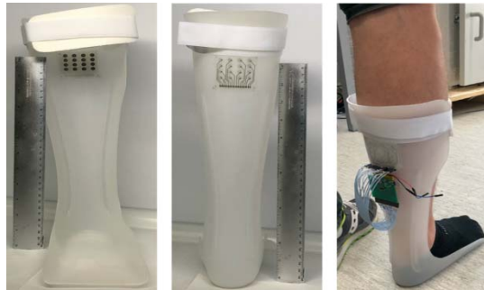
Fig. 2. Electrodes and tracks printed on the orthosis; a tester wearing the devices with the electronics.
